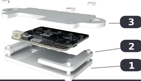
Stack each layer as numbered onto the screws through layer no. 1, then tighten nuts.
