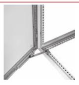
The Door Stop Kit holds doors open at 130 degrees. The kit includes a slotted bracket that mounts to either the top or bottom of the door and a stop arm that attaches to the frame. The Door Stop Kit is plated, mounts without drilling and includes all necessary mounting hardware. Not suitable for use with 180-degree hinging. Drill points in window door brackets for mounting Door Stop Kit.
