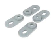
One-piece mounting foot kit consists of the necessary hardware to attach two fiberglass feet, molded from the same material as our A48 enclosure. This compression-molded fiberglass material has excellent chemical and temperature resistance and provides outstanding performance and durability in harsh environments. The mounting feet can be field installed on either the 18x16 or the 20x16 enclosure.
