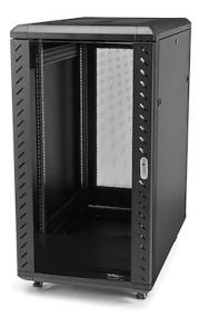
This server rack provides 25U of storage space in a sleek secure cabinet for storing EIA-310 compliant 19" rackmount devices such as Dell, HP and IBM servers along with telecommunication and A/V equipment. The rack creates a robust storage solution supporting a total load capacity of 800 kg. (1763.7 lbs.).
