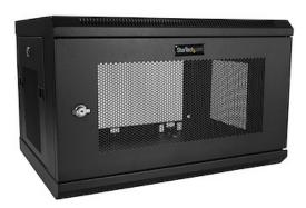
This 6U server rack cabinet lets you mount your EIA-310 compliant equipment to the wall. The enclosure features a mounting depth up to 15 in. and offers a maximum load capacity of 200 lb. (90 kg).
