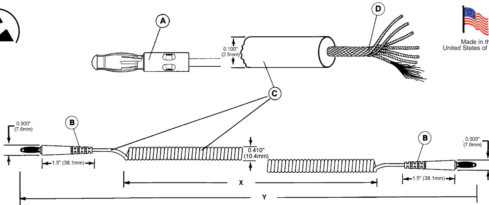
Banana-Banana Coil Cord allows cart users to ground carts to common grounding point on a bench.
