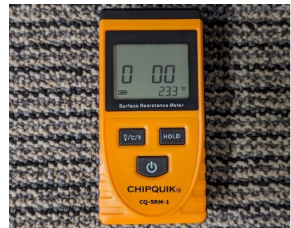
Image 3: Resistance on non-treated carpet (not conductive, not static dissipative)
