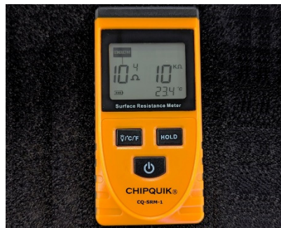
Image 2: Resistance on black ESD foam (conductive)
