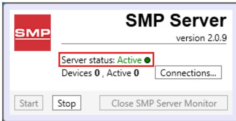
7. SMP Server will search and find the Ground Master Monitor on the network. The Device and Active counts will increase to 1.
