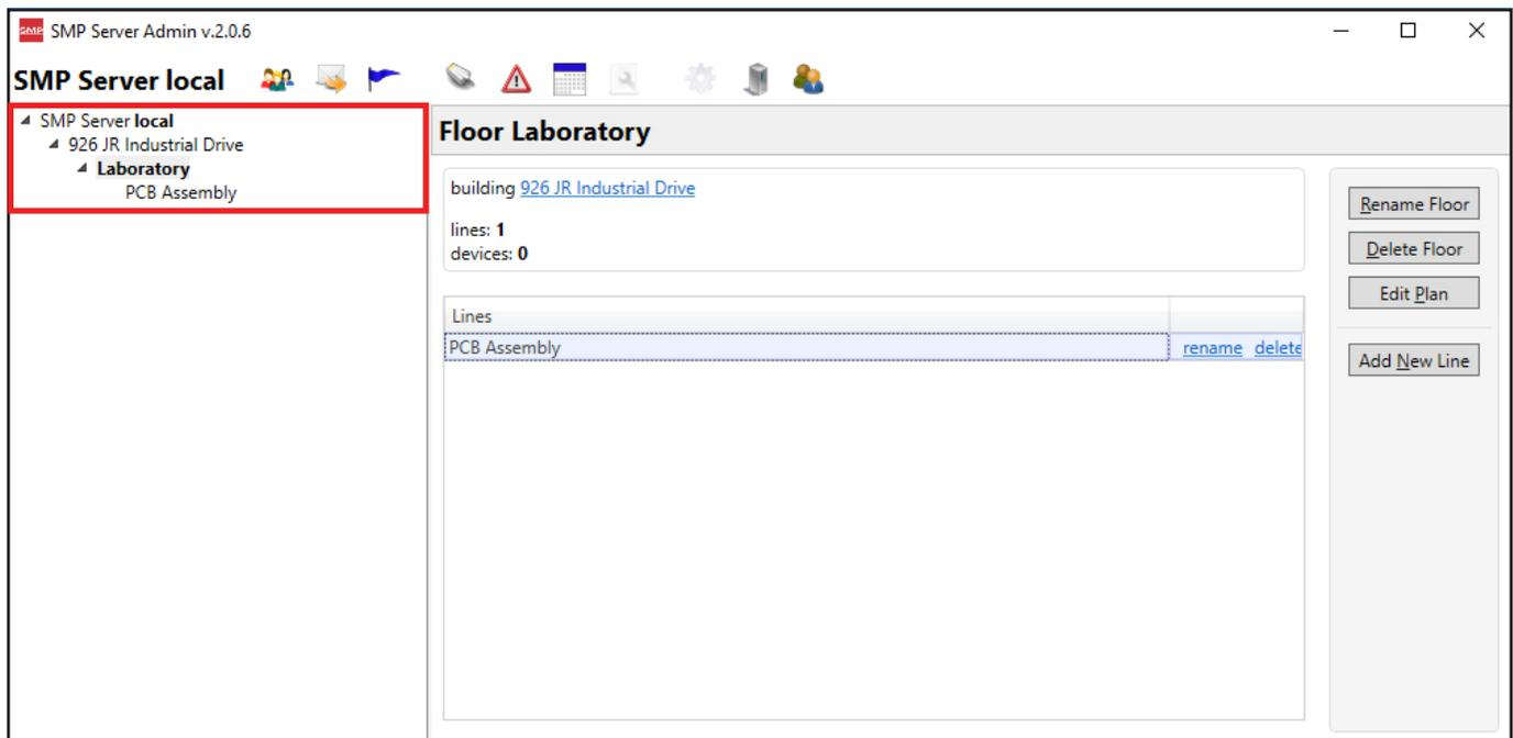
18. Click on the line name in the navigation pane, and then click the Attachable Devices arrow located at the bottom of the window.
