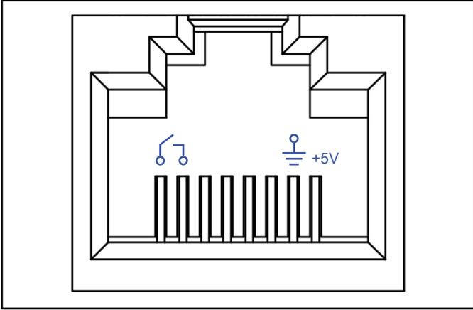
Figure 5. Relay terminal pin-out
