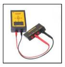
Verify the calibration of the SRM200 with the Veribox Decade Box. Resistance decade boxes can quickly and accurately simulate resistance for quickly testing the accuracy of ESD testers and meters.
