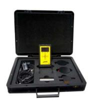
The measurements can be performed either with the built-in measurement electrodes on the underside of the instrument, with external probes such as the **SR400 Miniprobe** or the **SR820 Lightweight Travel Electrodes**. Performed measurements with external measuring electrode meet the requirements of ANSI/ESD STM4.1, ANSI/ESD STM7.1, ANSI/ESD STM7.1, ANSI/ESD STM12.1
