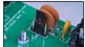
Figure 8. 220 VAC jumper setting
