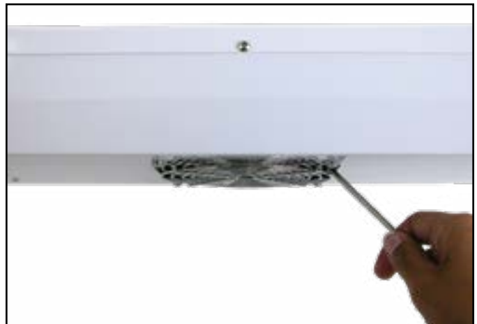
Figure 10. Shorting the ionizer's two fan grills
