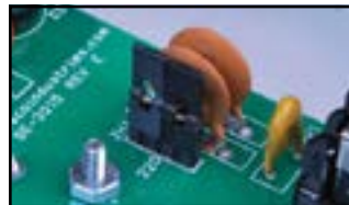
Figure 7. 120 VAC jumper setting
