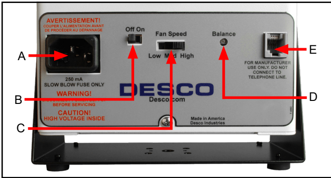
Figure 2. High Output Benchtop Ionizer features and components
