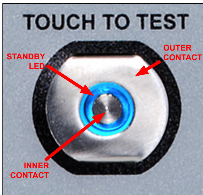
Figure 10. Steady-State Test Switch features and components
