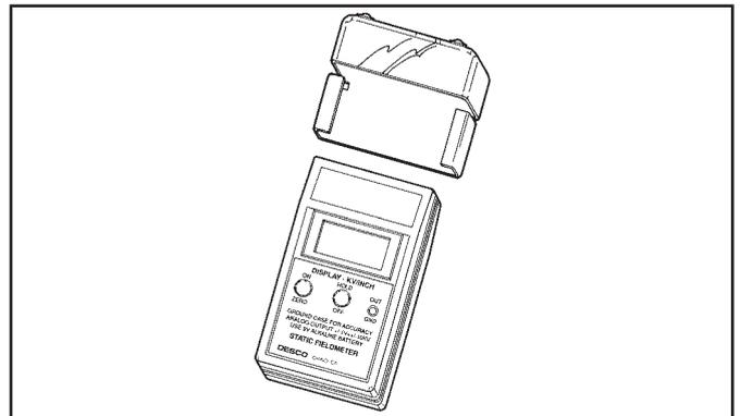
Figure 2. Installing the isolated plate assembly on the 19445 Digital Fieldmeter
