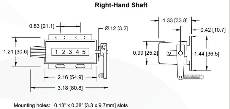
A highly versatile, 5 figure stroke counter. Numbers are large and distinctive for easy viewing, even when above or below eye level. Ruggedly built for years of trouble-free use. An excellent choice for counting parts produced.
