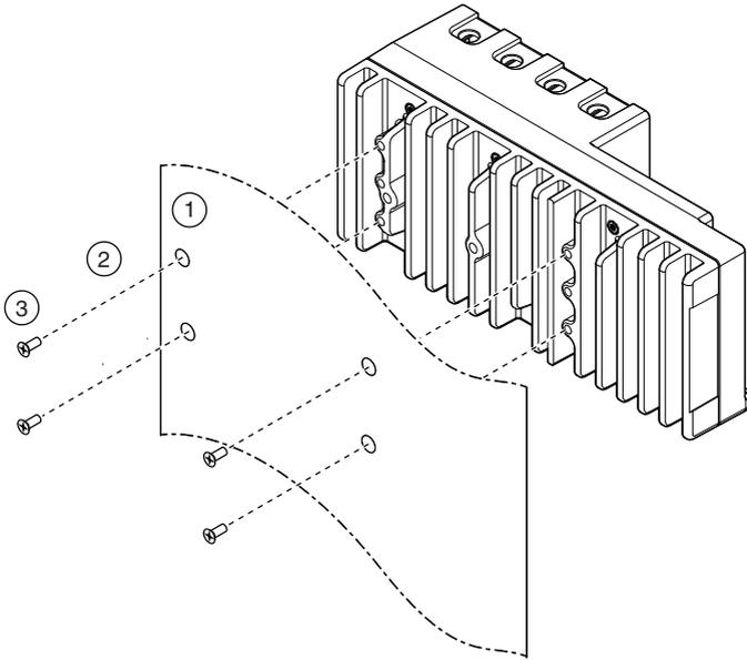
**Figure 15. Rear Mounting the 8-slot cRIO-905x Directly on a Flat Surface**
