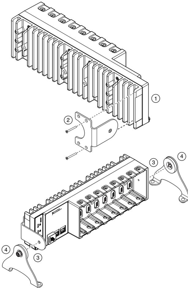
1. Use the Torx T10 screwdriver to remove the two screws from the back of the chassis on the controller side.
