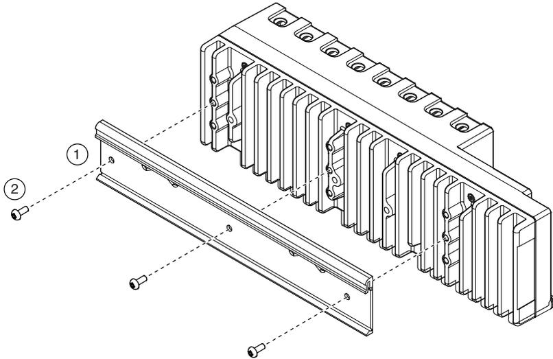
1. Align the DIN rail clip with the mounting holes on the rear of the cRIO-905x.
