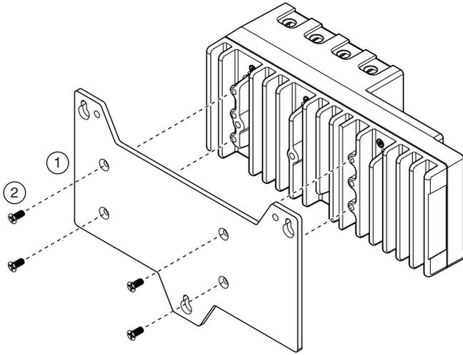
**Figure 23.** Mounting the 8-slot cRIO-905x on a Panel
