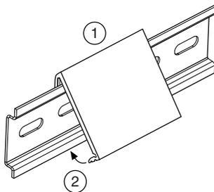
1. Latch the spring side (top) of the DIN clip onto the top edge of the DIN rail.
