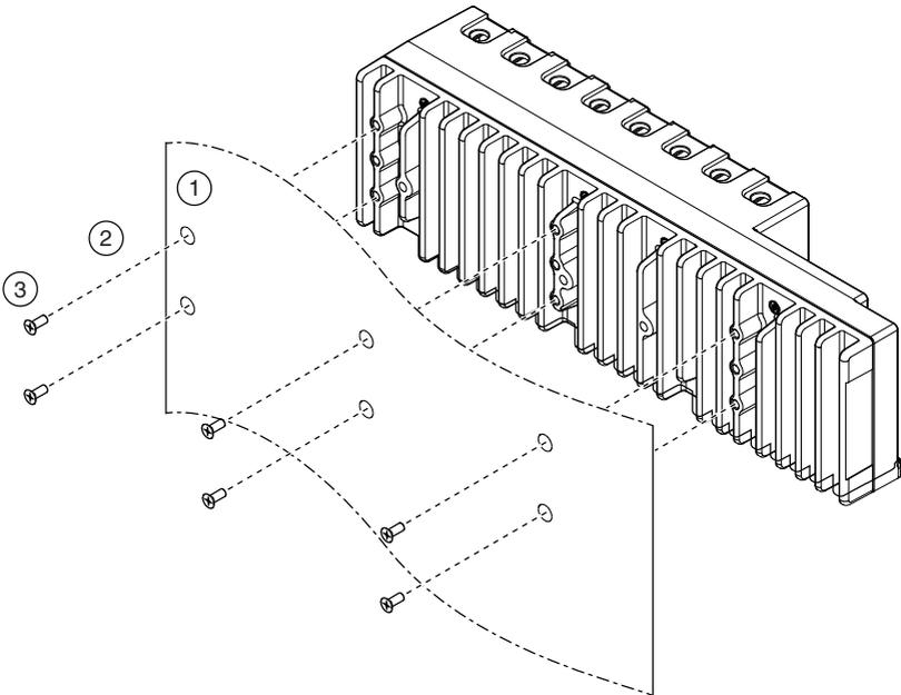
1. Prepare the surface for mounting the cRIO-905x using the *Surface Mounting Dimensions*.
