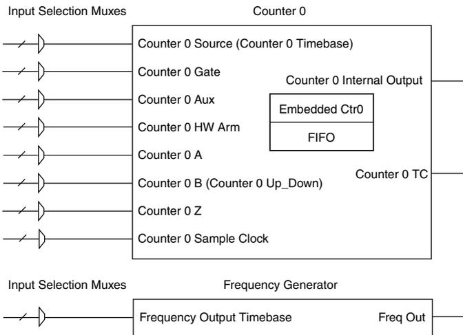
Counters have eight input signals, although in most applications only a few inputs are used.
