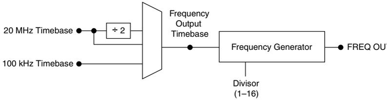
The frequency generator generates the Frequency Output signal. The Frequency Output signal is the Frequency Output Timebase divided by a number you select from 1 to 16. The Frequency Output Timebase can be either the 20 MHz Timebase, the 20 MHz Timebase divided by 2, or the 100 kHz Timebase.
