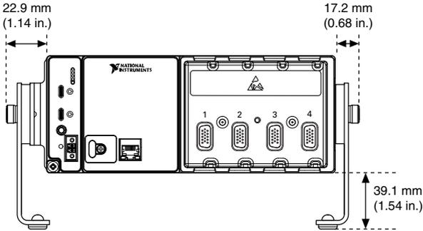
**Figure 33.** 8 Slot cRIO-905x Desktop Mounting Front Dimensions
