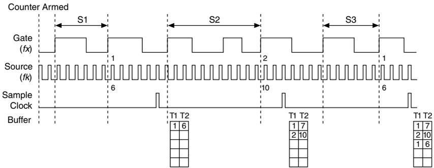
When **CI.Freq.EnableAveraging** is set to False, the frequency measurement returns the frequency of the pulse just before the sample clock. This single measurement is a single frequency measurement and is not an average between clocks as shown in the following figure.
