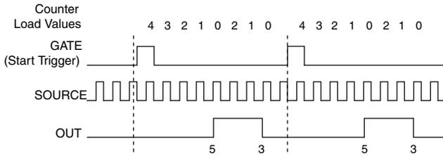
The figure below shows the same pulse train with **CO.EnableInitialDelayOnRetrigger** set to the default False.
