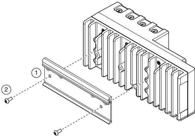
**Figure 27.** Mounting the 8-slot cRIO-905x on a DIN Rail
