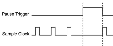
If you are using any signal other than the onboard clock as the source of the sample clock, the generation resumes as soon as the pause trigger is deasserted and another edge of the sample clock is received, as shown in the figure below.
