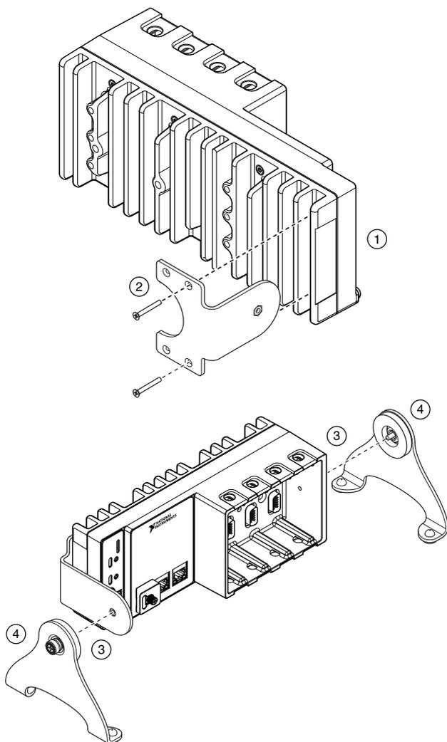
**Figure 31.** Mounting the 8-Slot cRIO-905x on a Desktop
