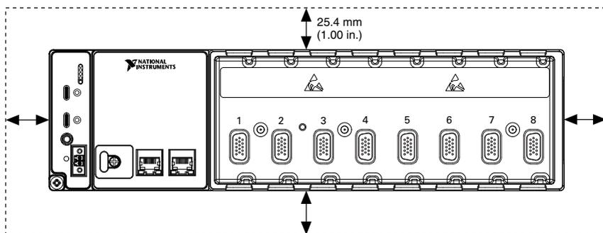
**Figure 9. Cabling Clearance**
