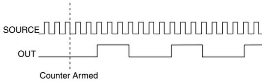
Continuous pulse train generation is sometimes called frequency division. If the high and low pulse widths of the output signal are  $M$  and  $N$  periods, then the frequency of the Counter  $n$  Internal Output signal is equal to the frequency of the Source input divided by  $M + N$ .
