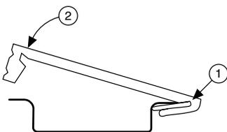
1. Insert one edge of the DIN rail into the deeper opening of the DIN rail clip.
