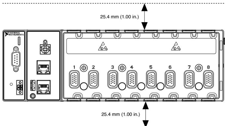
Allow the appropriate space in front of C Series modules for cabling clearance, as shown in the following figure. The different connector types on C Series modules require different cabling clearances. For a complete list of cabling clearances for C Series modules, visit [ni.com/info](http://ni.com/info) and enter the Info Code crioconn.
