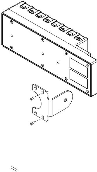
1. Use a #1 Phillips screwdriver to remove the two screws from the back of the chassis on the front-panel side.
