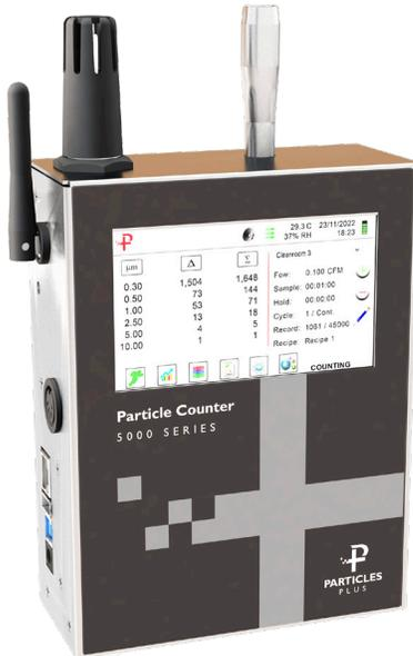
The Particles Plus® 5301P and 5501P Remote Particle Counters measure 0.3 or 0.5 to 25.0 µm and are the most feature advanced remote particle counters available. Integration is easy into a building automation and cleanroom management system via Ethernet, or (optional) Wireless 802.11 b/g, RS485 or RS232. Integrated web server displays instrument screen through any browser.
