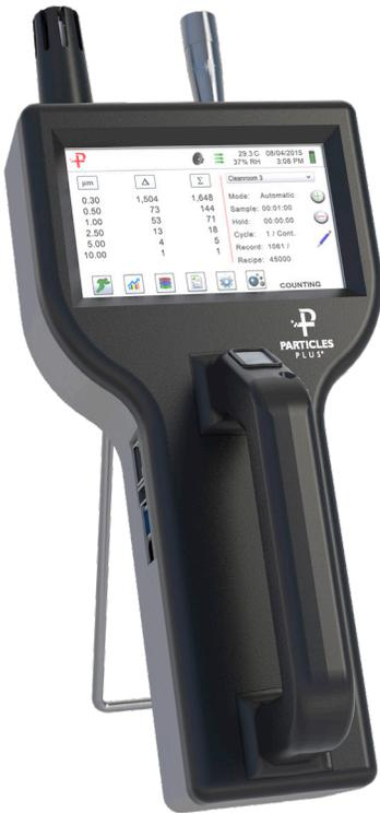
The Particles Plus® 8306 Handheld Particle Counter measures 0.3 to 25.0 µm with a flow rate of 0.1 CFM (2.83 LPM).
