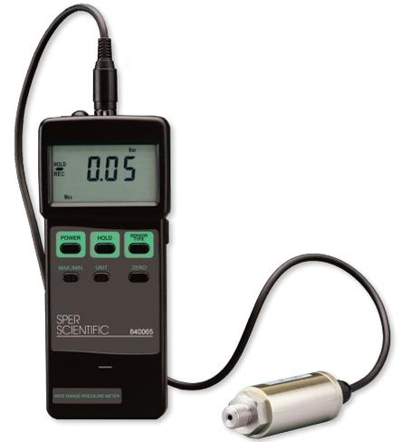
These pressure transducers come with the thread size of 1/4" NPT (per inch 18 teeth) and one adapter connector with the tread size of 1/4 inch PS (per inch 19 teeth). To use the 1/4" NPT threads directly, you will need to remove the adaptor connector from the transducer manually.
