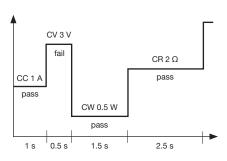
Execute multiple test sequences in automatic test mode. Up to 100 different sequences can be linked to run steps of various operating modes and load conditions.
