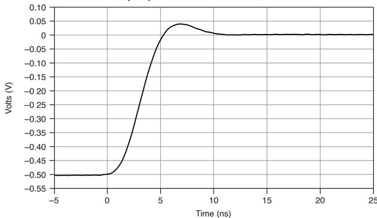
Figure 4. Step Response, 1 MΩ, 1 V<sub>pk-pk</sub>, 500 ps Rising Edge, Measured
