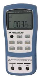
The Model 890B Capacitance Meter's large 4.5 digit LCD dual display can simultaneously display values and deviations from selected tolerances. The unit can also sort on preset tolerances of 1, 5, and 10%. The built-in chip and microprocessor allows the user to program unique values to sort specific circuit applications. Optional software and cabling is available for PC based data logging and monitoring via a USB interface.
