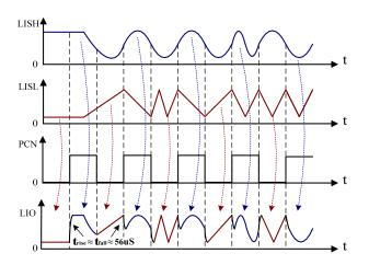
Figure 3. Digitally Controlled Analog Modulation Principle
