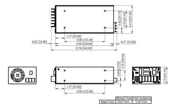
Figure 17. Mechanical Dimensions
