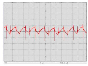
Figure 16. Noise Waveform at LDA Pin
