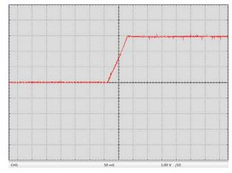
Figure 15. Start-up Waveform at LDA Pin
