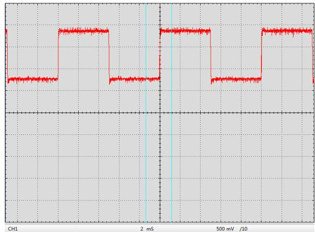
**Figure 8. Digital Modulation Response at LDA Pin**
