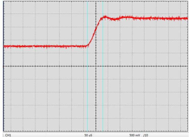
**Figure 7 . Digital Modulation Response at LDA Pin**
