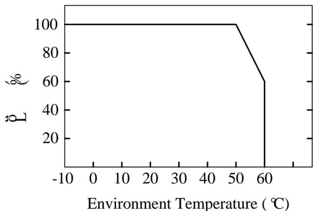
Figure 26. Derating Curve
