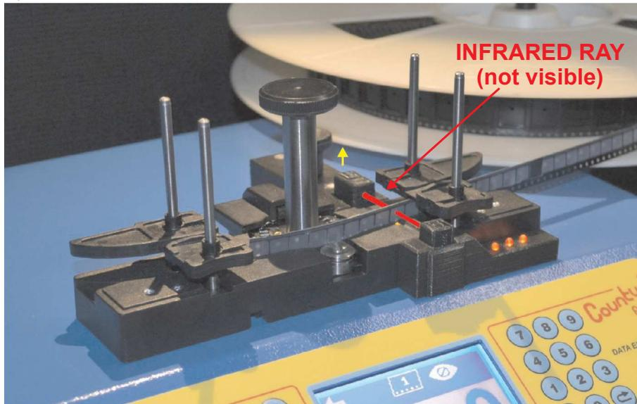
8) Turn the HEIGHT SETTING KNOB 360° clockwise (half turn) in order to give a better tolerance to the settings
