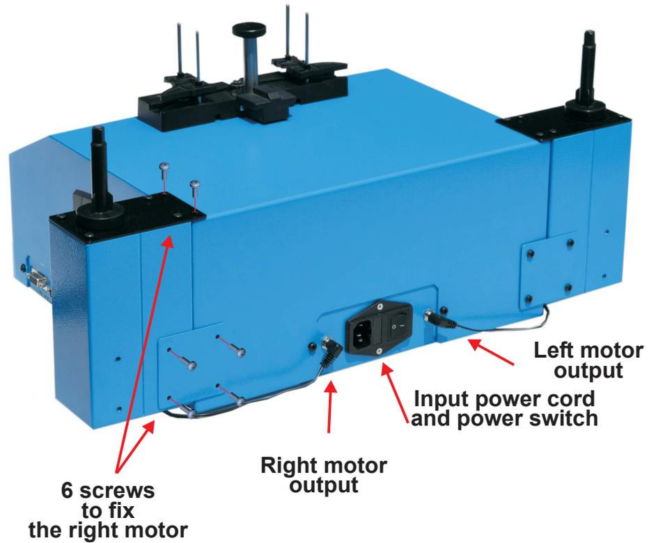
Screw the 2 groups using the 6 motor mounting screws (in the photo is shown the fixing of the right motor)
