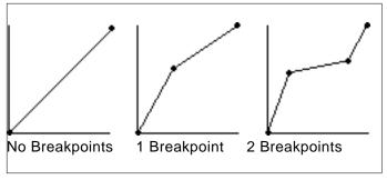
Figure 3. Piece-wise linear technique.
