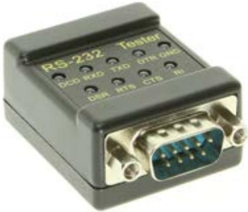
[DB9-TERS](#) is a RS-232 link tester. ASM232 can test the signal of PC to RS-232 Printer or RS-232 Terminate; It is standard DB-9 Male to DB-9 Female link tester. ASM-232 use 9 pcs LED to show the test result.
