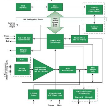
This block diagram shows all the subsystems and useraccessible signals of the DT9805 and DT9806 modules.
