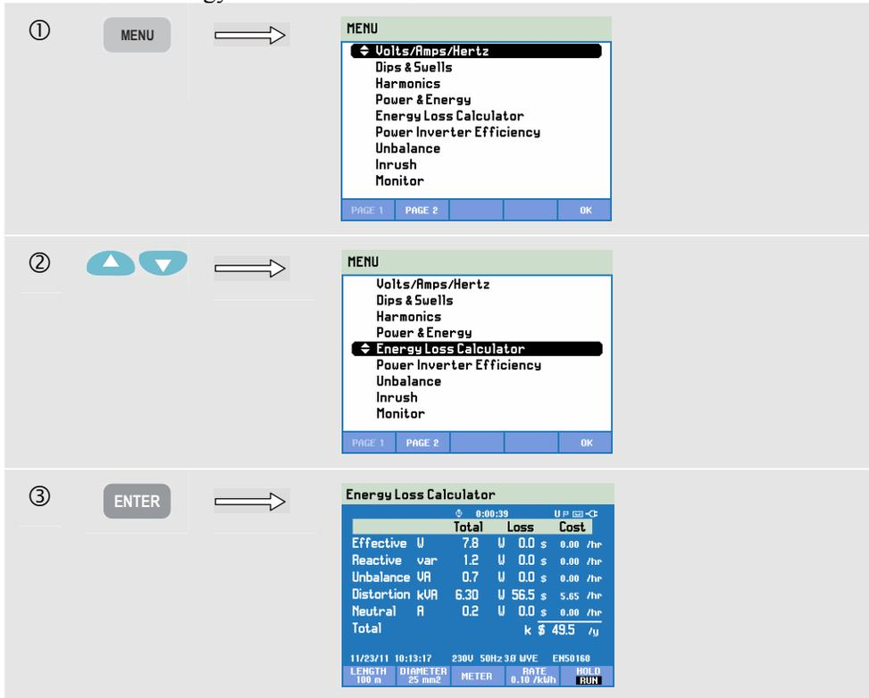
Cable properties, tariff and currency can be preset via the key sequence SETUP key, F4 – MANUAL SETUP, F3 – FUNCTION PReference, F4 – ENERGY LOSS. How to proceed is explained in Chapter 24 Setup.
