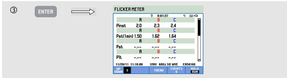
Flicker is characterized by: instantaneous flicker Pinst, short term severity Pst (measured over 1 min for fast feedback), short term severity Pst (measured over 10 min) and a long term severity Plt (measured over 2 hours). Also related data such as half cycle rms for voltage ( $V_{rms} \frac{1}{2}$ ), current ( $A_{rms} \frac{1}{2}$ ) and frequency are measured.
