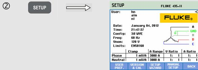
Press SETUP to access setup entry screen.
