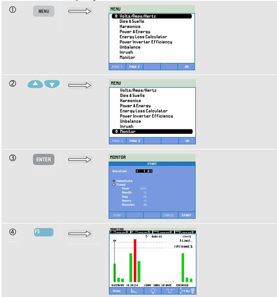
Power Quality Monitoring is reached via the MONITOR selection under the MENU key. A start menu allows for Immediate or Timed start. With the left/right arrow keys you can position the Cursor on a particular Bar Graph. Measuring data belonging to the bar is shown in the screen header.
