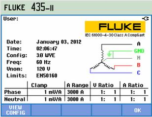
The active configuration is indicated in text and in a diagram behind Config.
