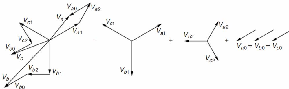
$$V_a = V_{a1} + V_{a2} + V_{a0}, \quad V_b = V_{b1} + V_{b2} + V_{b0}, \quad V_c = V_{c1} + V_{c2} + V_{c0}$$
