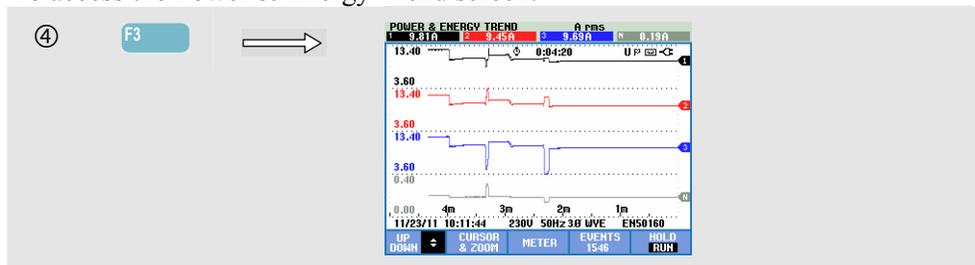
The figures in the Meter screen are instantaneous values that update constantly. Changes in these values over time are recorded whenever the measurement is active. All values in the Meter screen are recorded, but the Trends from each row in the Meter screen are displayed one at a time. The arrow keys are assigned to scroll the Trend screen.
