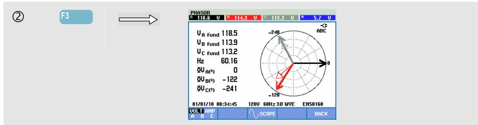
The Phasor screen displays the phase relation between voltages and currents in a vector diagram. The vector of reference channel A (L1) points in the positive horizontal direction. Additional numerical values are fundamental phase voltage and/or current, frequency, and phase angles. The screen header shows rms voltage and/or current values.
