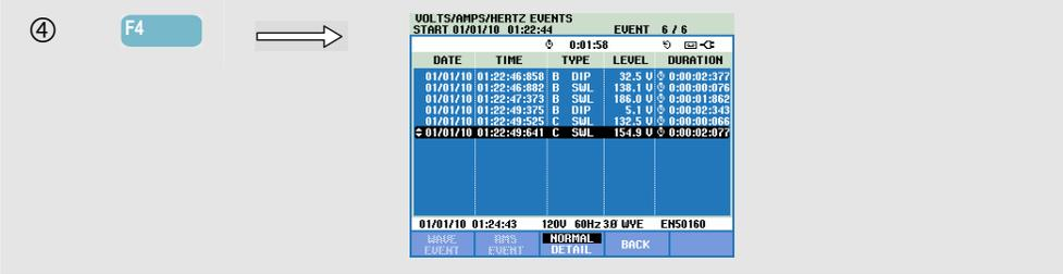
The Events table lists all threshold crossings of phase voltages. Thresholds according to international standards or user-definable thresholds can be used. Threshold adjustment is reached via the SETUP key and Limits. For detailed information see Chapter 24, Limits Adjustments.
