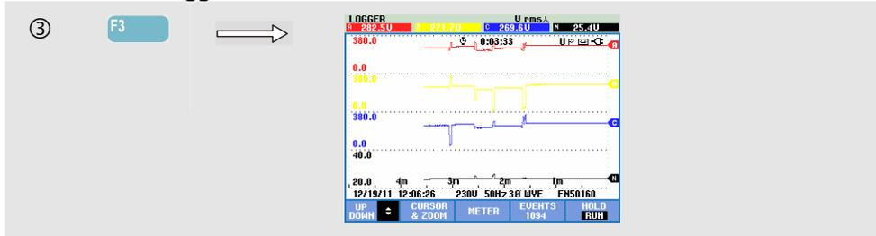
All readings are recorded during logging, but not all of them are visible at a time. Use the up/down arrow keys to make the desired set of trends visible within the viewing area.
