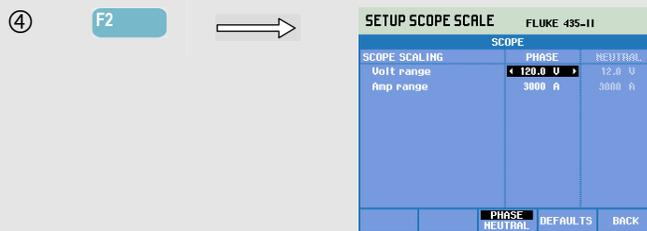
Press function key F2 to access Scope display scaling.
