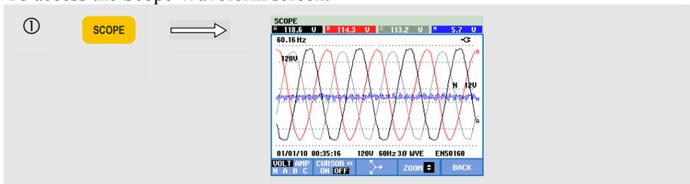
The Scope Waveform screen offers an oscilloscope style of display of voltage and/or current waveforms with a fast update rate. The screen header shows the related rms voltage/current values (10/12 cycle rms or 150/180 cycle rms). Four waveform periods are displayed. Channel A (L1) is the reference channel.
