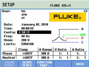
Return to Setup entry screen. The new configuration is indicated behind Config. and the belonging configuration symbol is shown on the right side of the screen.
