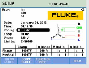
Note that a setup parameter is highlighted. If required use the up and down arrow keys to select setup parameter Config.
