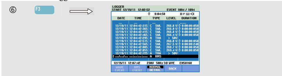
The Events table lists all threshold crossings of phase voltages. Thresholds according to international standards or user-definable thresholds can be used. Threshold adjustment is reached via the SETUP key and Limits. For detailed information see Chapter 24, Limits Adjustments.
