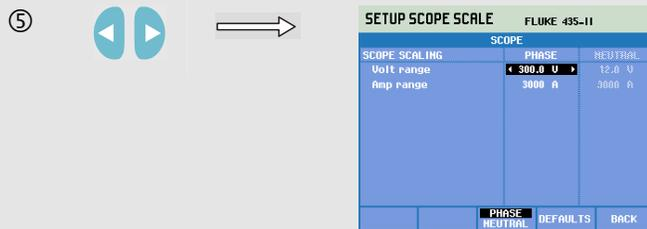
Use the left/right arrow keys to increase (e.g. to 300 V) the Voltage range of the Scope display.
