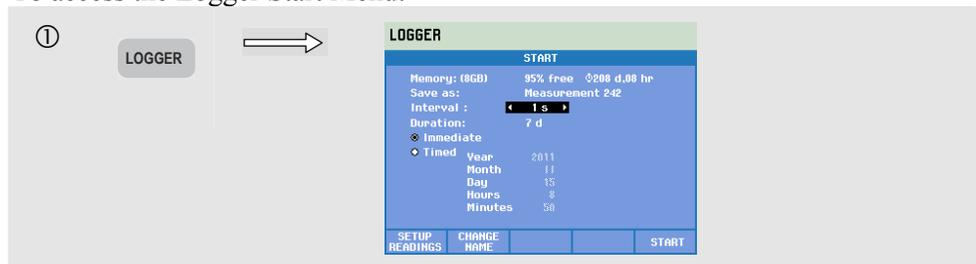
The set of readings to be logged is selectable in the menu under function key F1 – SETUP READINGS. The reading selection list for default frequency 50/60 Hz and 400 Hz are different. If you change the default frequency to 400 Hz or from 400 Hz to 50/60 Hz the reading selection list will be set to default!
