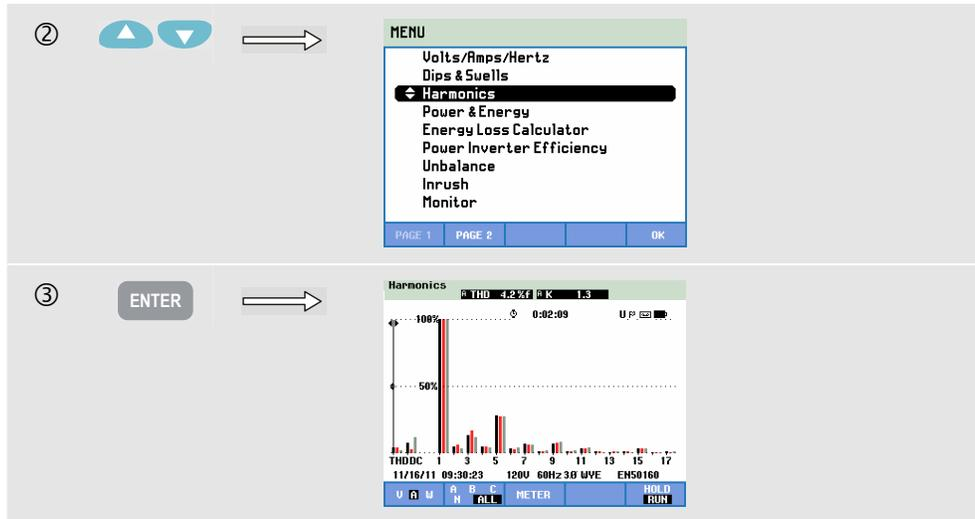
The Bar Graph display shows the percentage contribution of each of the components related to the full signal. A signal without distortion should show a 1<sup>st</sup> harmonic (= the fundamental) at 100 % while the others are at zero: in practice this will not occur because there always is a certain amount of distortion resulting in higher harmonics.
