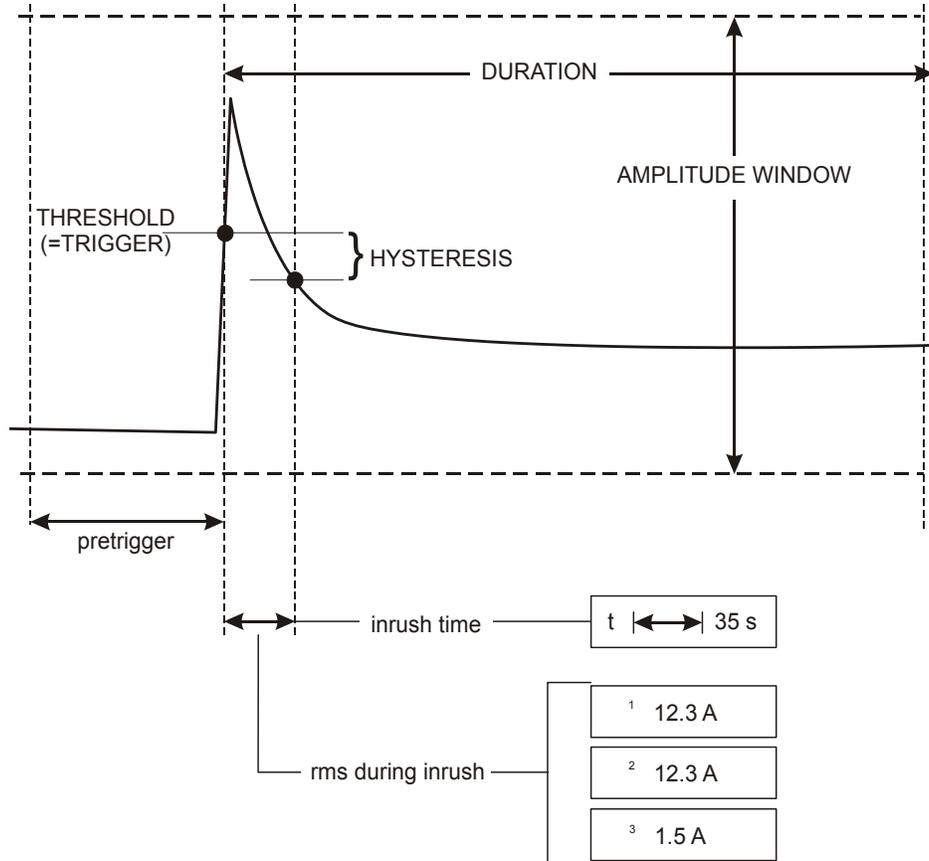
**Figure 15-1. Inrush characteristics and relation with start menu**
