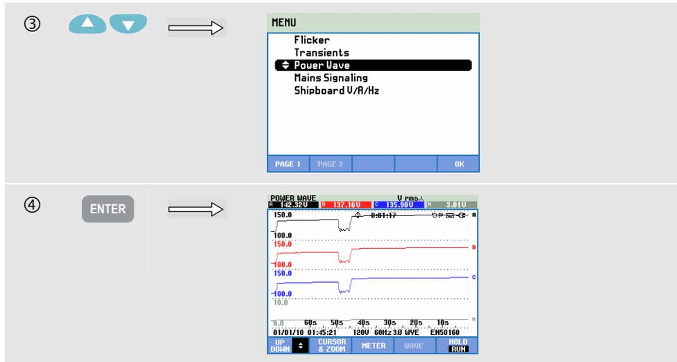
The traces build up from the right side. Readings in the header correspond to the most recent values plotted on the right. With the up/down arrow keys you can select all available trends.
