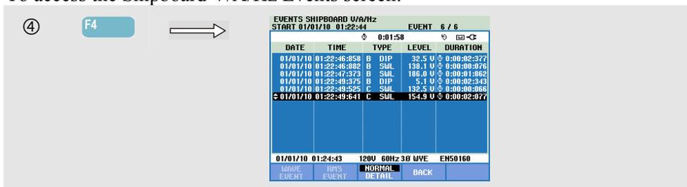
The Events table lists all threshold crossings of phase voltages. Thresholds according to international standards or user-definable thresholds can be used. Threshold adjustment is reached via the SETUP key and Limits. For detailed information see Chapter 23, Limits Adjustments.
