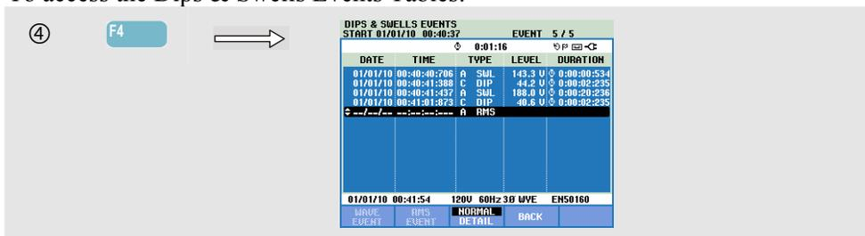
The Events table lists all threshold crossings of phase voltages. Thresholds according to international standards or user-definable thresholds can be used. Threshold adjustment is reached via the SETUP key, F4 – MANUAL SETUP and Limits. For detailed information see Chapter 24, Limits Adjustments.
