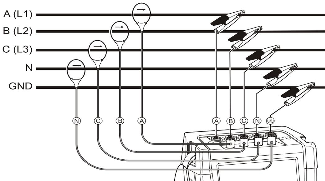
Figure 6-2. Connection of Analyzer to 3-phase distribution system
