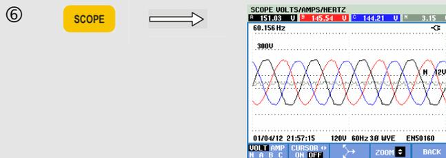
Return to the Scope display: the voltage waveforms of the Phases are inside the viewing window.
