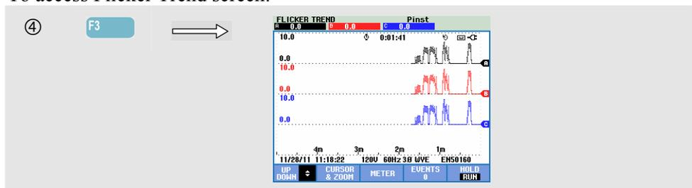
The parameters in the Meter screen update over time. They are recorded whenever the measurement is on. Trend displays the changes in these values over time. All values in the Meter screen are recorded, but the Trends from each row in the Meter screen are displayed one at a time. The arrow keys are assigned to scroll the trend screen. The Trend display may consist of 6 screens.
