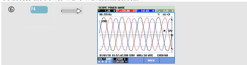
Starting from the Trend screen, position the cursor on the area of interest. Then press F4 – WAVE to open waveform display at this area.
