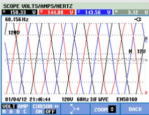
The voltage waveforms of the Phases are outside the viewing window.
