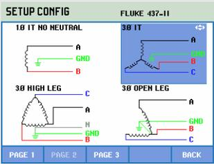
Use the arrow keys to highlight 3 $\phi$  IT. Then press ENTER to confirm the selection.
