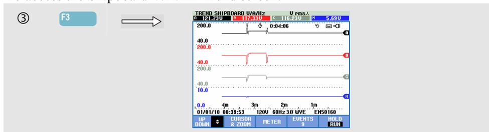
All values in the Meter screen are recorded, but the Trends from each row in the Meter screen are displayed one at a time. Press Function key F1 to assign the up/down arrow keys to row selection.
