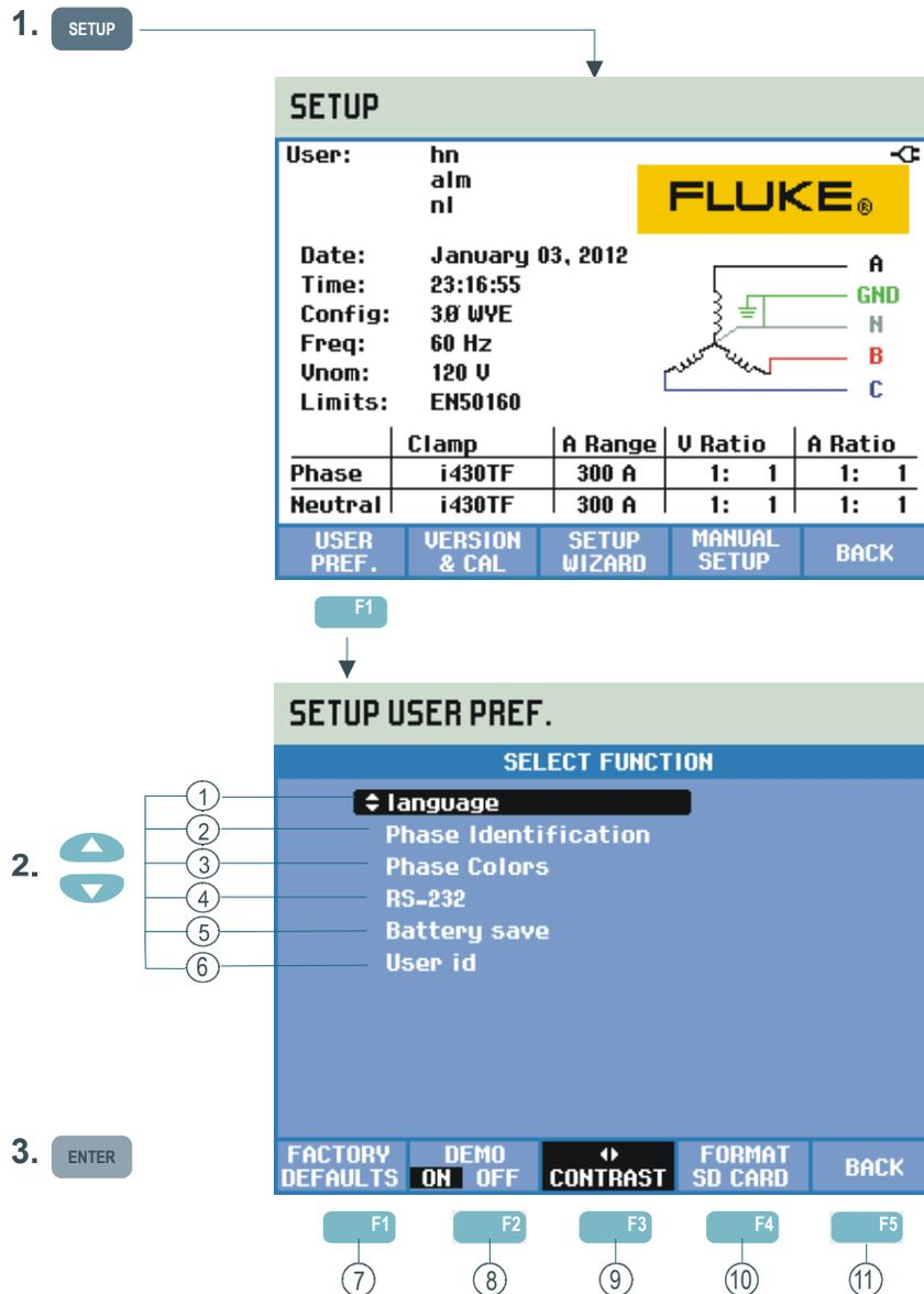
USER PReferences allows you to customize Information Language, Phase Identification, Phase Colors, RS-232 baudrate settings, Auto shut-off of display backlight, programming of User name/address (as shown in entry screen), Reset of Analyzer to Factory Defaults, Demo Mode on/off, display contrast, and clearing of memories.
