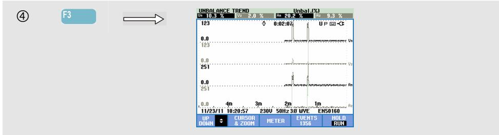
The figures in the Meter screen are instantaneous values that update constantly. Changes in these values over time are recorded whenever the measurement is active. All values in the Meter screen are recorded, but the Trends from each row in the Meter screen are displayed one at a time. Press function key F1 to assign the arrow keys to row selection. The Trend display may consist of 6 screens.
