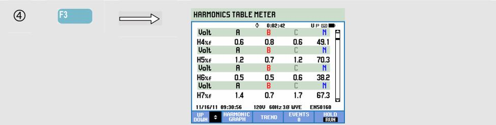
The Meter screen display shows many measurements that are grouped per phase. Use the up/down arrow keys to scroll all measurements within the viewing area.
