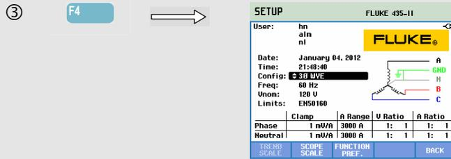
Press function key F4 to access the Manual Setup screen.
