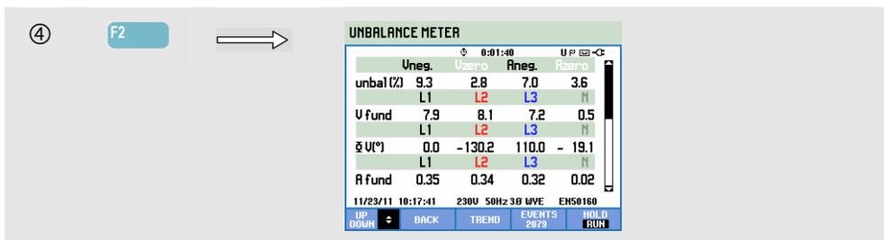
The Meter screen shows all relevant numerical values: negative voltage unbalance percentage, zero sequence voltage unbalance percentage (in 4-wire systems), negative current unbalance percentage, zero sequence current unbalance percentage (in 4-wire systems), fundamental phase voltage, frequency, fundamental phase current, angle between phase-neutral voltages relative to the reference phase A/L1 and angles between voltage and current for each phase.
