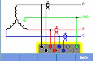
The diagram shows in detail how to connect voltage and current probes to the power system under test.
