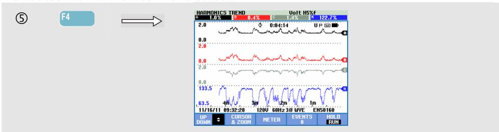
Trend shows how harmonics and related parameters vary over time: Cursor and Zoom can be used in HOLD mode to investigate trend details. All values in the Meter screen are recorded, but the Trends from each row in the Meter screen are displayed one at a time. Use the arrow keys to scroll the Trend screen.
