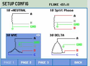
The screen shows 4 wiring configurations; 3-phase WYE IT configuration is not among them. Press F2 to access a second screen with 4 other configurations.
