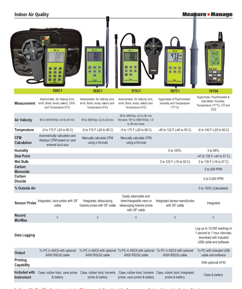
Indoor Air Quality Instruments to Measure: Airflow, Humidity, Temperature, Carbon Monoxide, Carbon Dioxide
