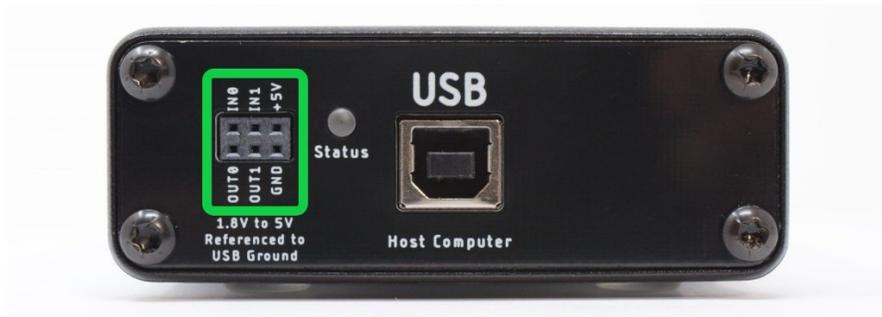
These signals enable time-synchronization with the device under test and other external equipment. The user interface can display GPIs time-synchronized with current, voltage, and power in the oscilloscope view.
