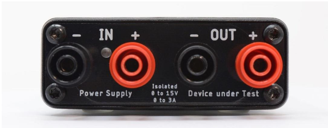
The LED indicates when your Joulescope is ready to collect measurements.
