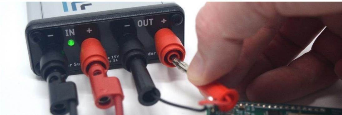
Operate your device under test. The Joulescope host software starts in the **Multimeter** view by default. Use the **Multimeter** view to measure the current, voltage, power, charge, and energy consumption.
