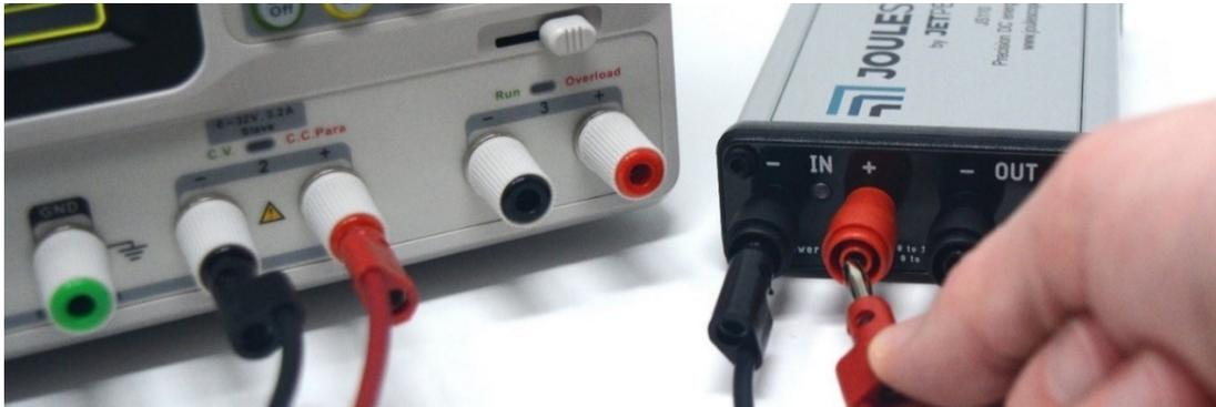
Connect the Joulescope “OUT” port to the power input for your device under test.
