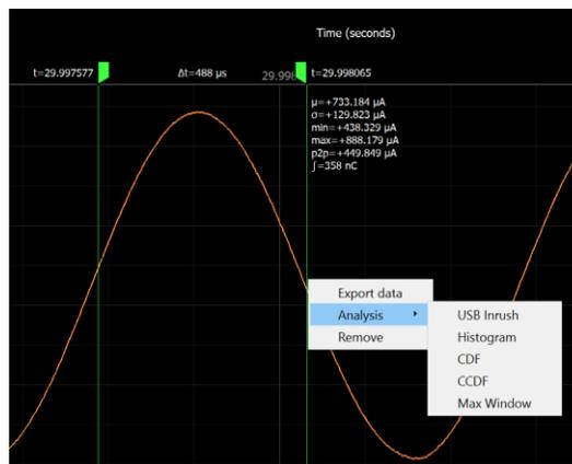
Use the scroll wheel to zoom in and zoom out. The zoom operation keeps the point under the mouse cursor at the same location after the zoom operation. However, when you reach the maximum extents while zooming out, that point may move. When viewing live data, the zoom operation always keeps the most recent data in view at the right.
