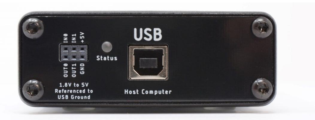
Use the provided USB cable to connect the USB host computer connector to your host computer. The status LED indicates when the Joulescope successfully communicates with the host computer. For Windows hosts, the Status LED illuminates shortly after connecting the Joulescope to the computer. For Linux and macOS hosts, the Status LED will not illuminate until the Joulescope software attempts to connect.
