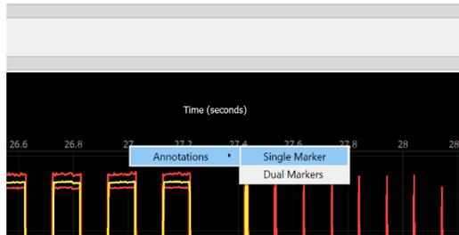
Left-click the marker to move it with the mouse. As you move the mouse over the waveforms, the vertical marker follows along. The line displays statistics about that location:
