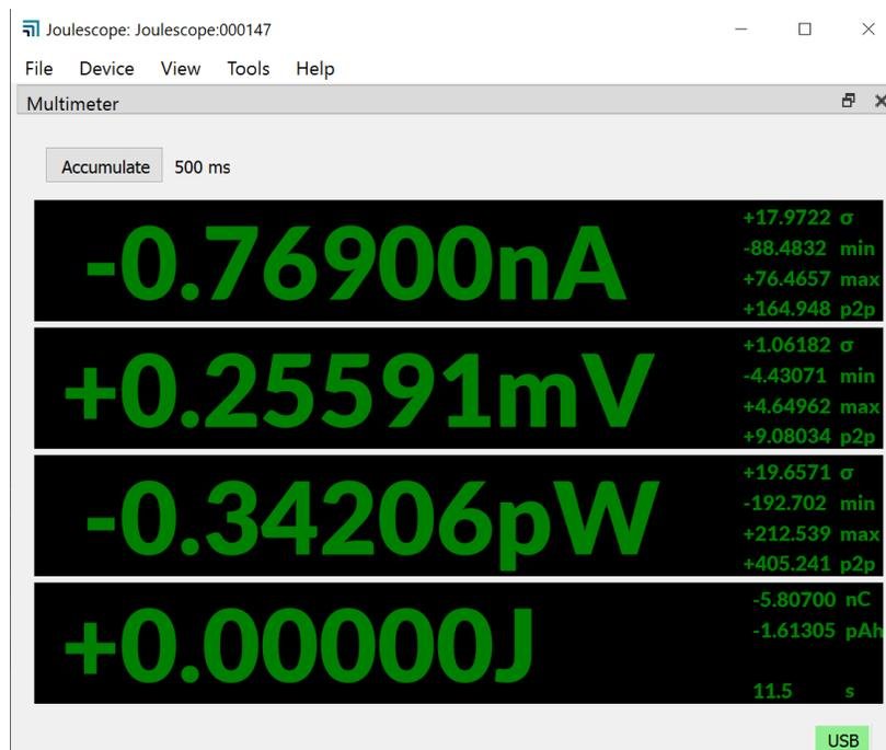
Connect the Joulescope **IN** port to your power source. If using a configurable power supply, set the voltage and current suitable for your device under test. The maximum voltage between **IN+** and **IN-** should never exceed  $\pm 15V$ . **IN** and **OUT** are electrically isolated from USB, but the voltage between any port and USB ground should never exceed  $\pm 48V$ .
