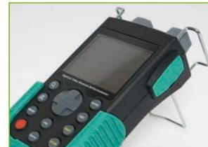
Adjustable back tilt device with hook-up
