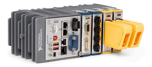
C Series Functional Safety modules can connect to sensors or final elements and allow for fast safety response that meets the demands of the process industry and production engineering.
