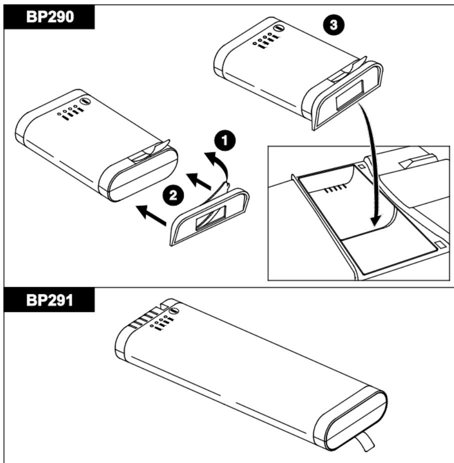
The BP291 does not need any modification before you install the battery pack into the test tool.
