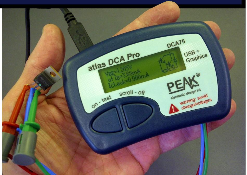
Detailed component information on your PC, complete with curve tracing functions.
