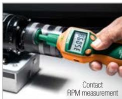
Contact RPM measurement
