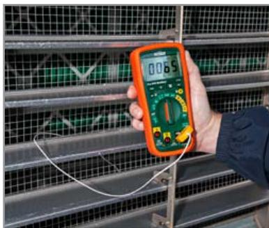
Verify Temperature output on HVAC units using Model EX355
