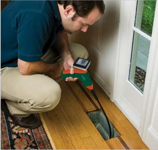
**3.5" Color Detachable Wireless LCD Monitor can be viewed from a remote location up to 32 ft (10 m) from measurement point**
