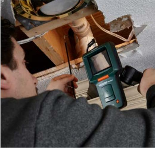
**Articulating (240°) camera tip facilitates viewing in obstructed areas where standard camera tips cannot access**
