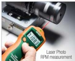
Laser Photo RPM measurement
