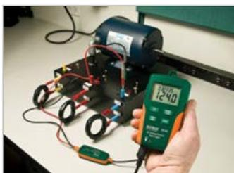
Datalogs up to 100,000 readings with programmable sample rate from 1 sec to 24 hrs
