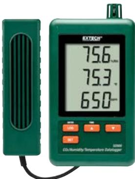
Includes sensor with 11.4" (290 mm) cable (wired to meter), 6 AAA batteries, SD memory card, Universal AC adaptor, and mounting bracket; 2-year warranty
