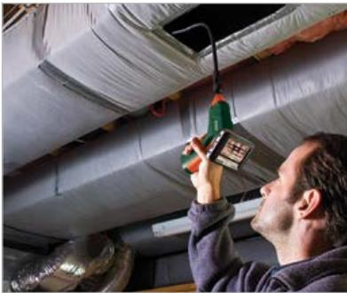
**9 mm camera diameter and 2.4" Color TFT LCD Monitor with video output for viewing on any monitor with a video input jack**
