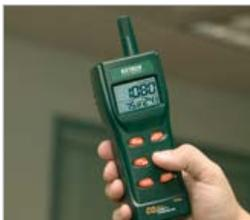
Measure CO<sub>2</sub> level in office buildings to ensure proper ventilation.
