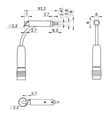
MA009068 is a highly durable test plug for testing optical TOSLINK connector interface. It has a TOSLINK jack with 1mm fibre cable for easy integration. Lenght of cable is 300mm.
