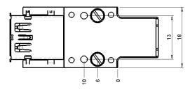
MA033469 USB3 Type-A Test Connector is a 9-pin Test Plug with straight signaling. It is also compatible with USB 2.0 type-A.
