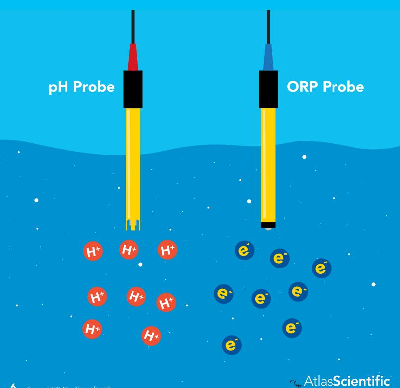
When reading the ORP of a liquid that has very few electrons available for transfer ORP readings can appear to be inconsistent.
