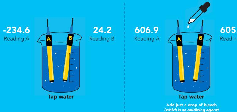
An ORP probe has a platinum tip that is connected to a silver wire, surrounded by silver chloride. That silver wire is then connected to a KCL reference solution. Because platinum is an unreactive metal it can "silently observe" the electron activity of the liquid without becoming apart of whatever reaction is occurring in the liquid.
