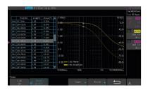
Bode Plot – The T3DSO1000 can control the USB AWG module, to scan an object's amplitude and phase frequency response, and display the data as a Bode Plot (not available on the T3DSO1102).
