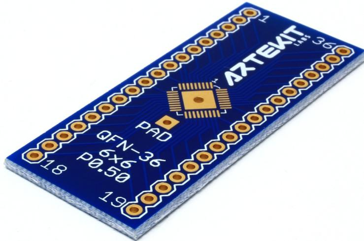
This adapter breaks out the pins of a QFN-36 component (with a body of 6mm x 6mm and 0.50mm pin pitch) into a board with 0.1" (2.54mm) spaced pins.
