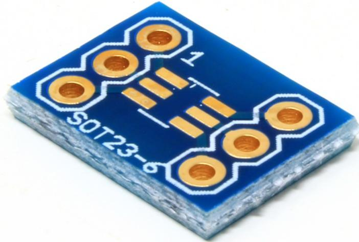
This adapter breaks out the pins of a SOT23-6 component (with 0.95mm pin pitch) into a board with 0.1" (2.54mm) spaced pins.
