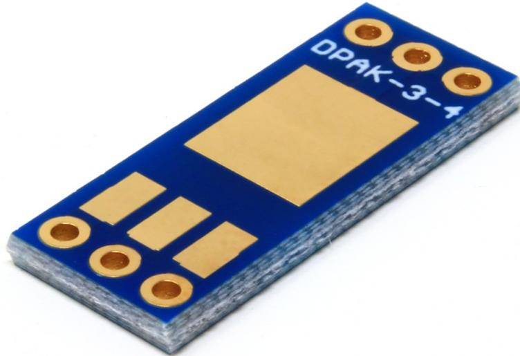
This adapter breaks out the pins of a component with TO252 package (also known as DPAK with 3 or 4 pins) into a board with 0.1" (2.54mm) spaced pins.
