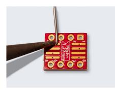
5. To be sure the IC gets flat against the PCB, first add heat to the solder you placed before, then solder the far pin to keep it stable.
