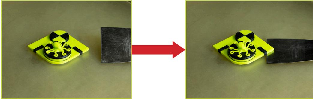
**!** *If using a sharp object, exercise caution when using it. The blade can cut, gouge, or cause other damage to the print surface. Caution should also be exercised to avoid causing personal injury during the print removal process. Avoid prying prints up and away from the bed.*
