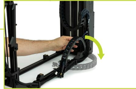
**i** If the Y-axis cable chain does not rotate back and downward easily, loosen the screw at the base of the cable chain to allow for easier adjustment.
