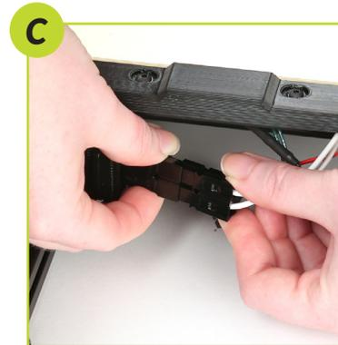
**!** Once all connections are in place, locate the bed power harness retention clip in your tool bag. Press the two prongs of the clip into the two holes on the heater connection.
