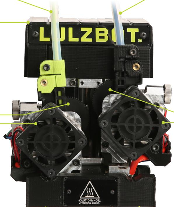
Extruder 2 Filament Guide Tube
