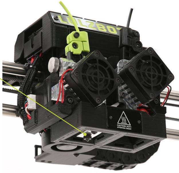
**5.4** Once the hot end reaches the appropriate filament removal temperature, press the **Continuous** button in the **Unload** column to start retracting filament. Once the filament stops moving, pull it out of the idler. Press the **Continuous** button again to stop the extruder. Select the **2 button** and repeat this process for **Extruder 2**.
