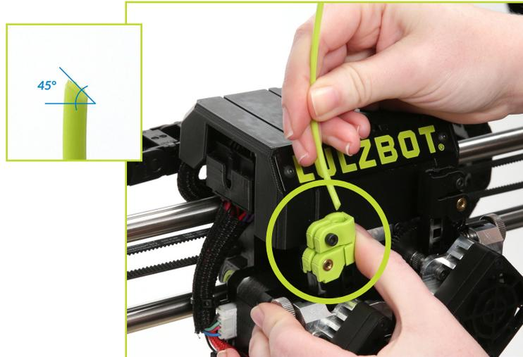
**5.11** Select **Extruder 1** and press the **Load/Extrude - Continuous** button and let filament advance until it extrudes smoothly and consistently as shown. Press the **Load/Extrude - Continuous** button again to stop extruding.
