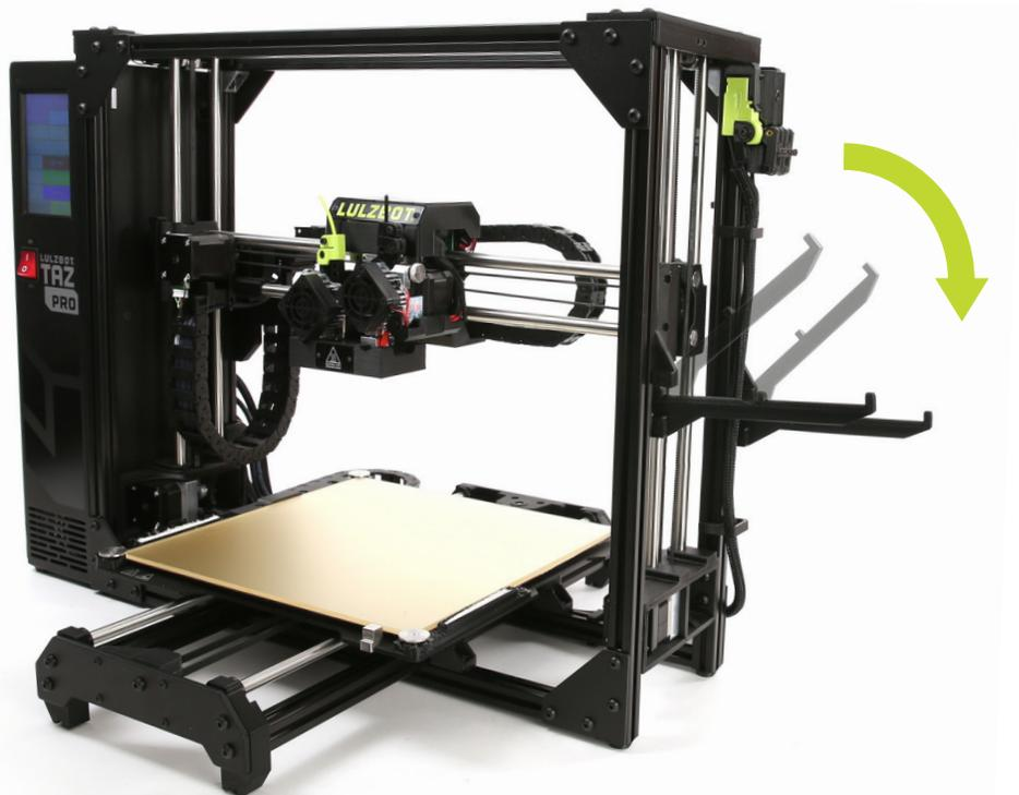
**5.b** Obtain the clear filament feed guide tubes for filament from the additional contents you removed from the box earlier. Insert the larger end of the feed guide into the top of the LulzBot Green filament sensor marked 1. Do the same with the black filament sensor marked 2.
