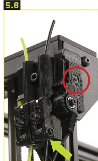
**i** Note that the filament sensors 1 and 2 correspond to Extruder 1 and Extruder 2 and must go to the correct extruder in order for your TAZ Pro to function properly.
