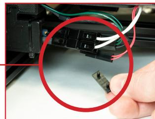
**3.9** Align the end of the Y-axis cable chain under the modular print bed as shown. Once in place, secure the cable chain to the bed using the included 4mm hex key and the **captive inset screw** on the modular print bed. Turn the 4mm hex key counter-clockwise until you feel the threads seat (to prevent stripping the threads), then while holding the cable chain level, turn the 4mm hex key clockwise to screw on the cable chain.
