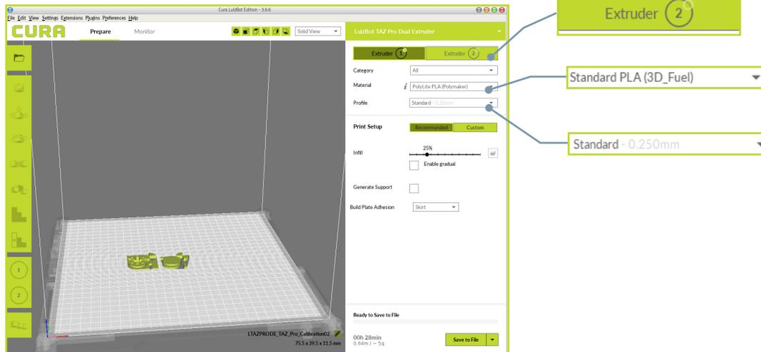
**4.7** Click on the **TAZ\_Pro\_Calibration02.stl** model on the virtual print bed, then click on the **2** on the left side of the print area. This designates **TAZ\_Pro\_Calibration02.stl** as the piece to be printed with the **Extruder 2**. The model with change color based on the filament selected for **Extruder 2** to reflect the change.
