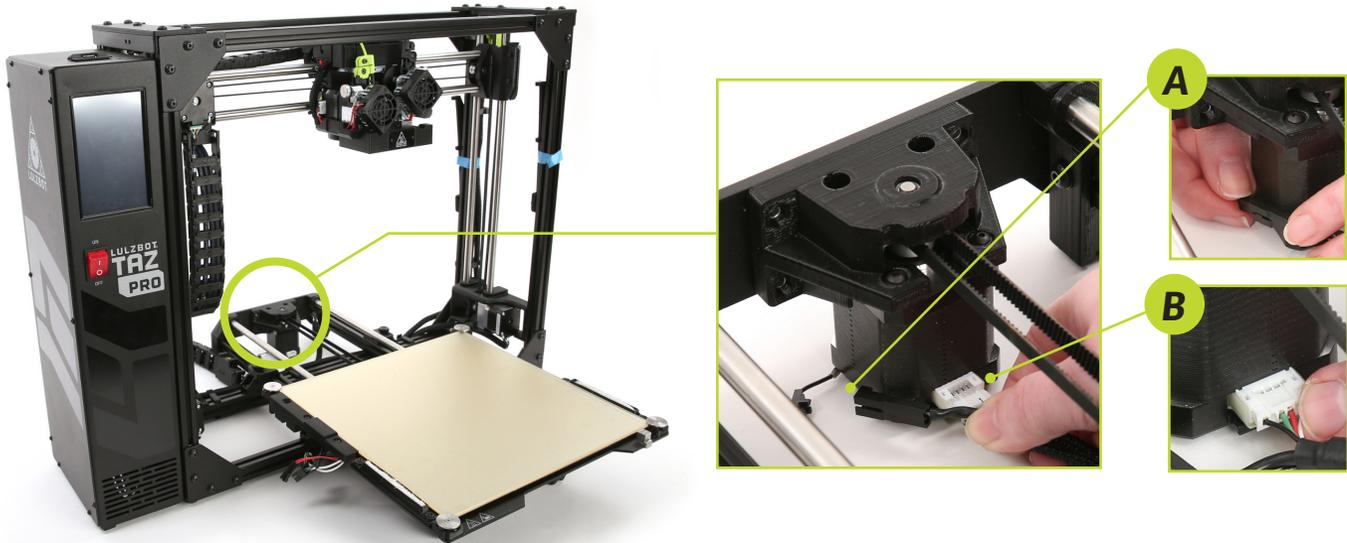
**3.7** **A** Connect the three sets of wire connectors underneath the bed as shown below, starting with the small two pin connection, **B** then the small three pin connection, **C** then the large heater connection.
