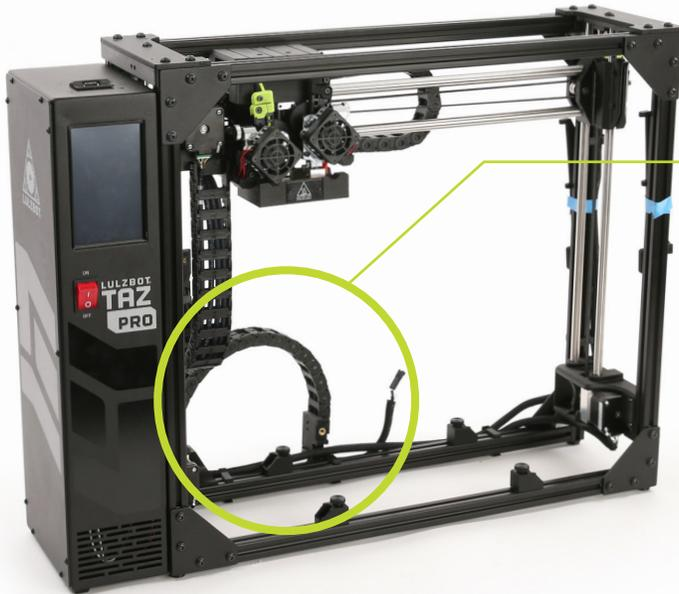
**3.2** Move the Y-axis cable chain into place by grasping the base of the cable chain and rotating it back and downward 90° away from the machine until it snaps into place.
