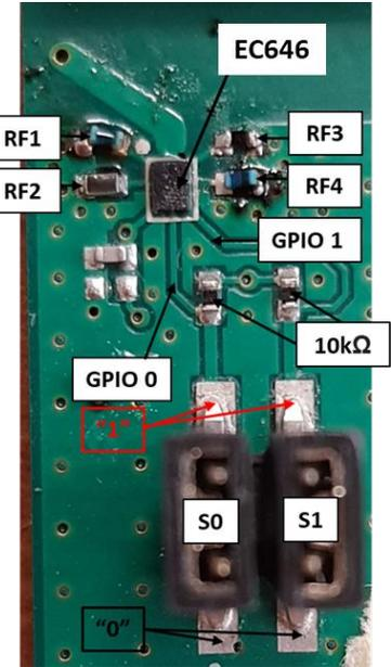
High and low state are controlled by connecting S0 or S1 with a 10kΩ resistor to either state “1” or state “0”.
