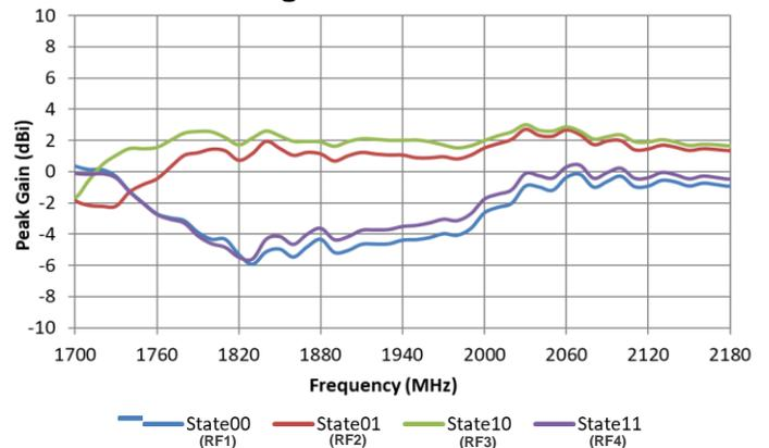
LTE Active Tuning Solution + switch KYOCERA AVX Demo Board Specifications
