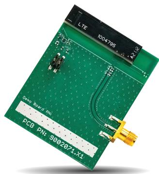
KYOCERA AVX Band Switching technology using standard products allows faster time-to-market. The Evaluation Board has a small size of 45.5 x 60 mm, which allows engineers test the antenna performance on a typical size of IoT devices, reducing the number of iterations and improving the accuracy.
