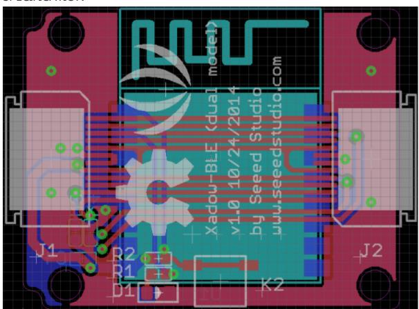
**K2:**During connected status,It would be disconnected by pressing K2 more than 100ms.During sleeping model,It could be restored through pressing K2 factory settings.
