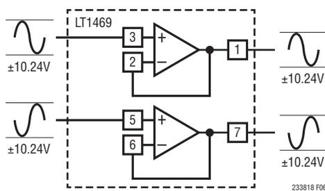
**Figure 6.** LT1469 Buffering a Fully Differential Signal Source
