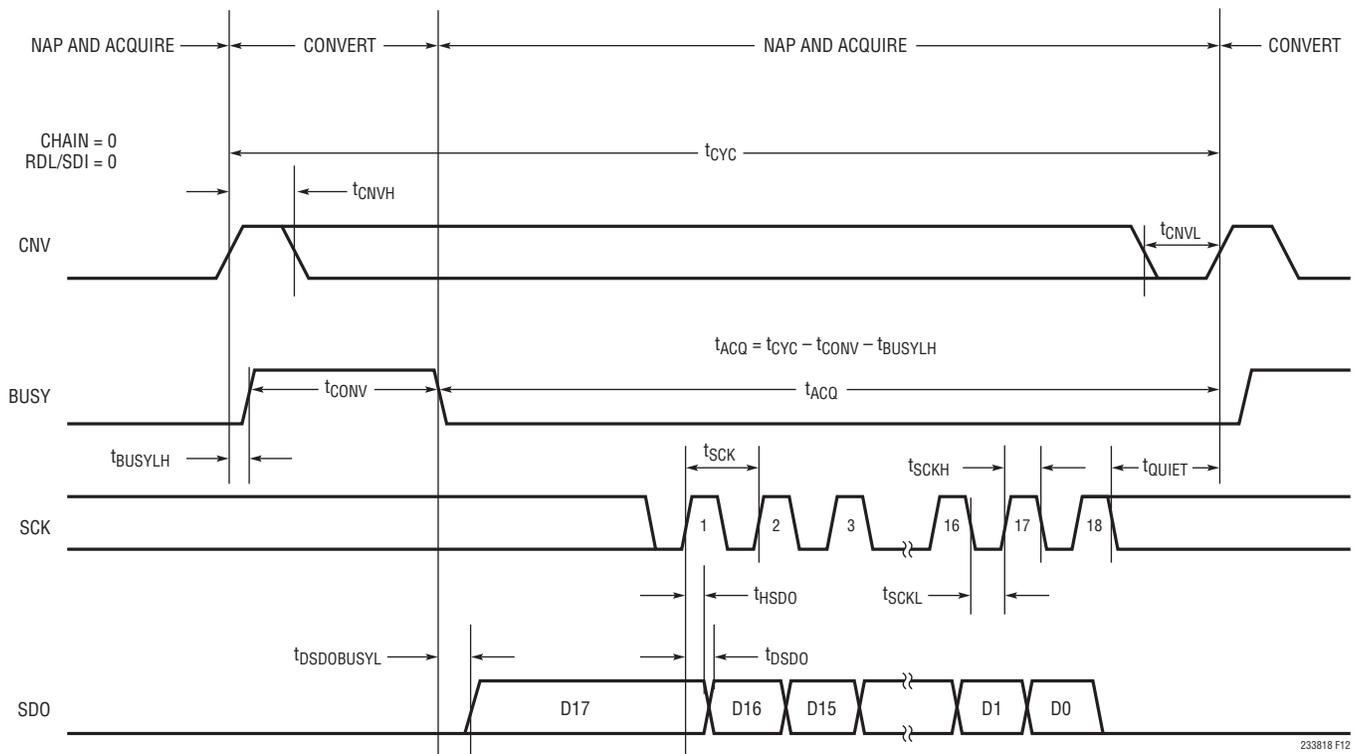
Figure 12. Using a Single LTC2338-18 in Normal Mode
