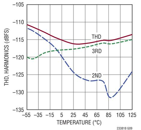
**TYPICAL PERFORMANCE CHARACTERISTICS**  $T_A = 25^\circ\text{C}$ ,  $V_{DD} = 5\text{V}$ ,  $OV_{DD} = 2.5\text{V}$ ,  $REF_{IN} = 2.048\text{V}$ ,  $f_{SAMPL} = 1\text{Msps}$ , unless otherwise noted.
