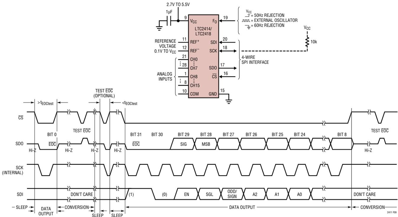
Figure 9. Internal Serial Clock, Reduced Data Output Length
