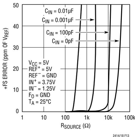
Figure 13. +FS Error vs R<sub>SOURCE</sub> at IN<sup>+</sup> or IN<sup>-</sup> (Small C<sub>IN</sub>)
