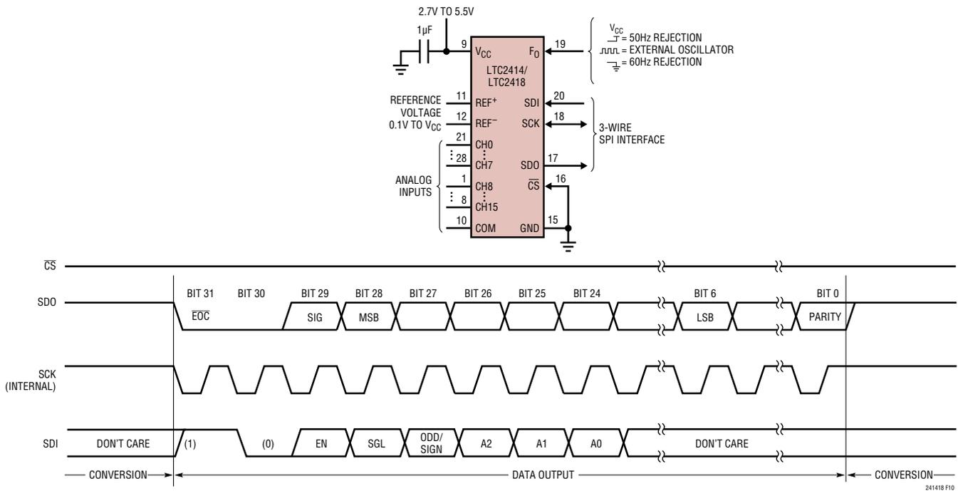
**Figure 10. Internal Serial Clock,  $\overline{CS} = 0$  Continuous Operation**
