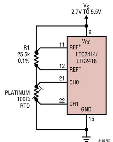
Figure 44. Remote Half Bridge Interface
