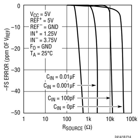
Figure 14. -FS Error vs R<sub>SOURCE</sub> at IN<sup>+</sup> or IN<sup>-</sup> (Small C<sub>IN</sub>)
