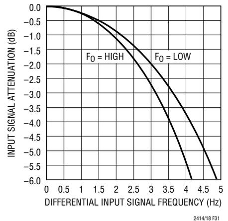
**Figure 31. Input Signal Bandwidth Using the Internal Oscillator**
