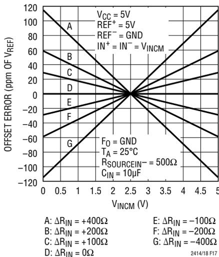
Figure 17. Offset Error vs Common Mode Voltage (V<sub>INCM</sub> = IN<sup>+</sup> = IN<sup>-</sup>) and Input Source Resistance Imbalance (ΔR<sub>IN</sub> = R<sub>SOURCEIN+</sub> - R<sub>SOURCEIN-</sub>) for Large C<sub>IN</sub> Values (C<sub>IN</sub> ≥ 1 μF)
