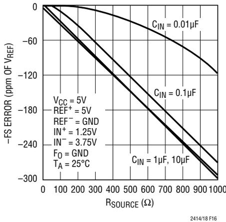
Figure 16. -FS Error vs R<sub>SOURCE</sub> at IN<sup>+</sup> or IN<sup>-</sup> (Large C<sub>IN</sub>)
