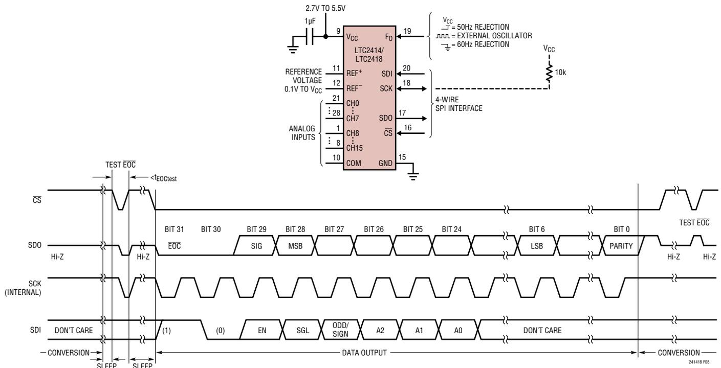
**Figure 8. Internal Serial Clock, Single Cycle Operation**
