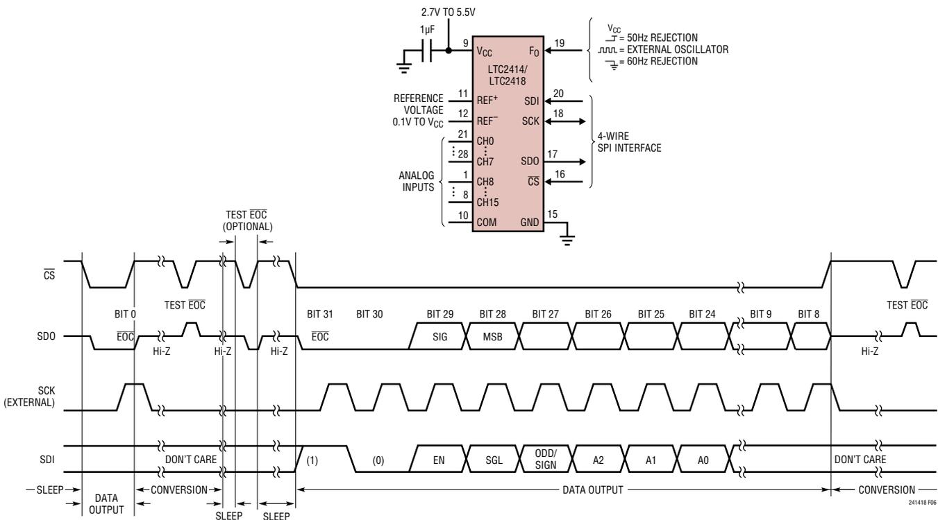
Figure 6. External Serial Clock, Reduced Data Output Length
