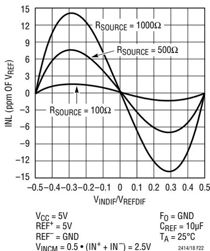
**Figure 22. INL vs Differential Input Voltage ( $V_{\text{IN}} = \text{IN}^+ - \text{IN}^-$ ) and Reference Source Resistance ( $R_{\text{SOURCE}}$  at  $\text{REF}^+$  and  $\text{REF}^-$  for Large  $C_{\text{REF}}$  Values ( $C_{\text{REF}} \geq 1\mu\text{F}$ )**
