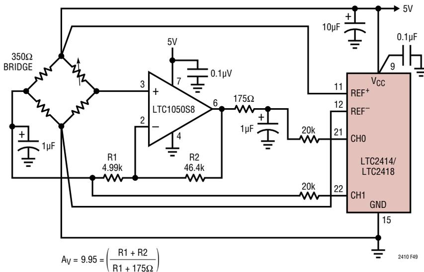
Figure 43. Bridge Amplification Using a Single Amplifier
