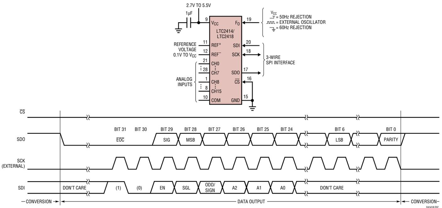
Figure 7. External Serial Clock,  $\overline{CS} = 0$  Operation
