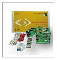
The kit is a development platform for the ATmega128RFA1 based pluggable radio modules deRFmega128-22A00 and deRFmega128-22A02 for the 2.4 GHz frequency band. It allows a quick start-up and tests of simple wireless radio applications based on the MAC stack or advanced development of own applications based on 6LoPWAN or ZigBee.
